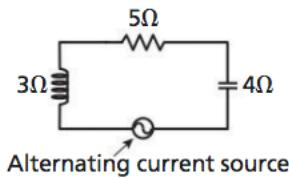
The table shows the relationship between a component's resistance or reactance and its contribution to impedance. A *series circuit* is also shown with the resistance or reactance of each component labeled. The impedance for a series circuit is the sum of the impedances for the individual components. Find the impedance of the circuit.
